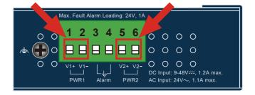
2. Tighten the wire-clamp screws for preventing the wires from loosening.
